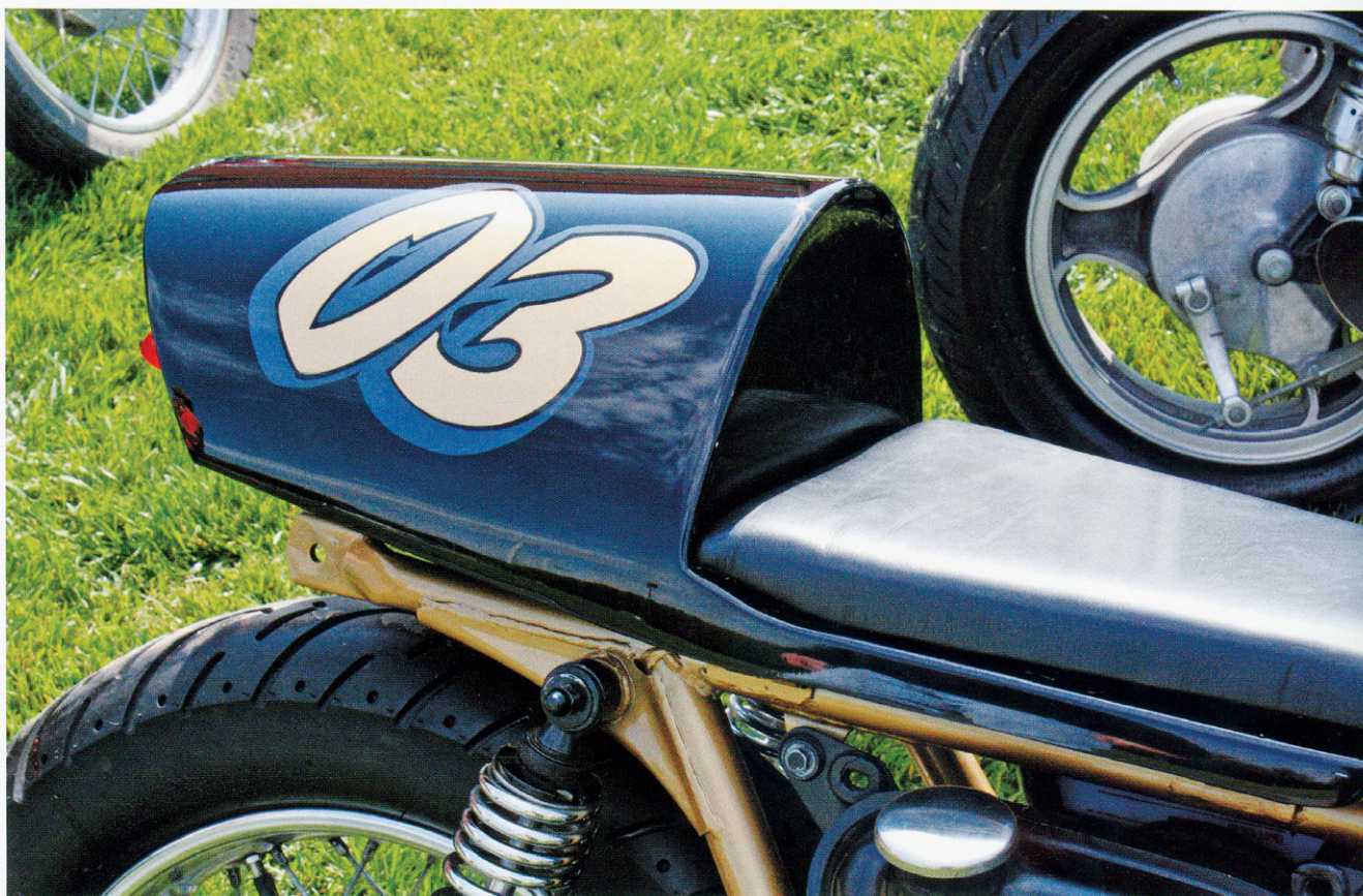
It's not automotive, but it's gorgeous. Ryan Brown made this handsome tail section for his Honda CB750 entirely with hand tools and the English wheel using principles you will learn in this chapter. Ryan's tail section boasts a subtle compound curve that both streamlines and enhances the otherwise chunky proportions of this motorcycle.
