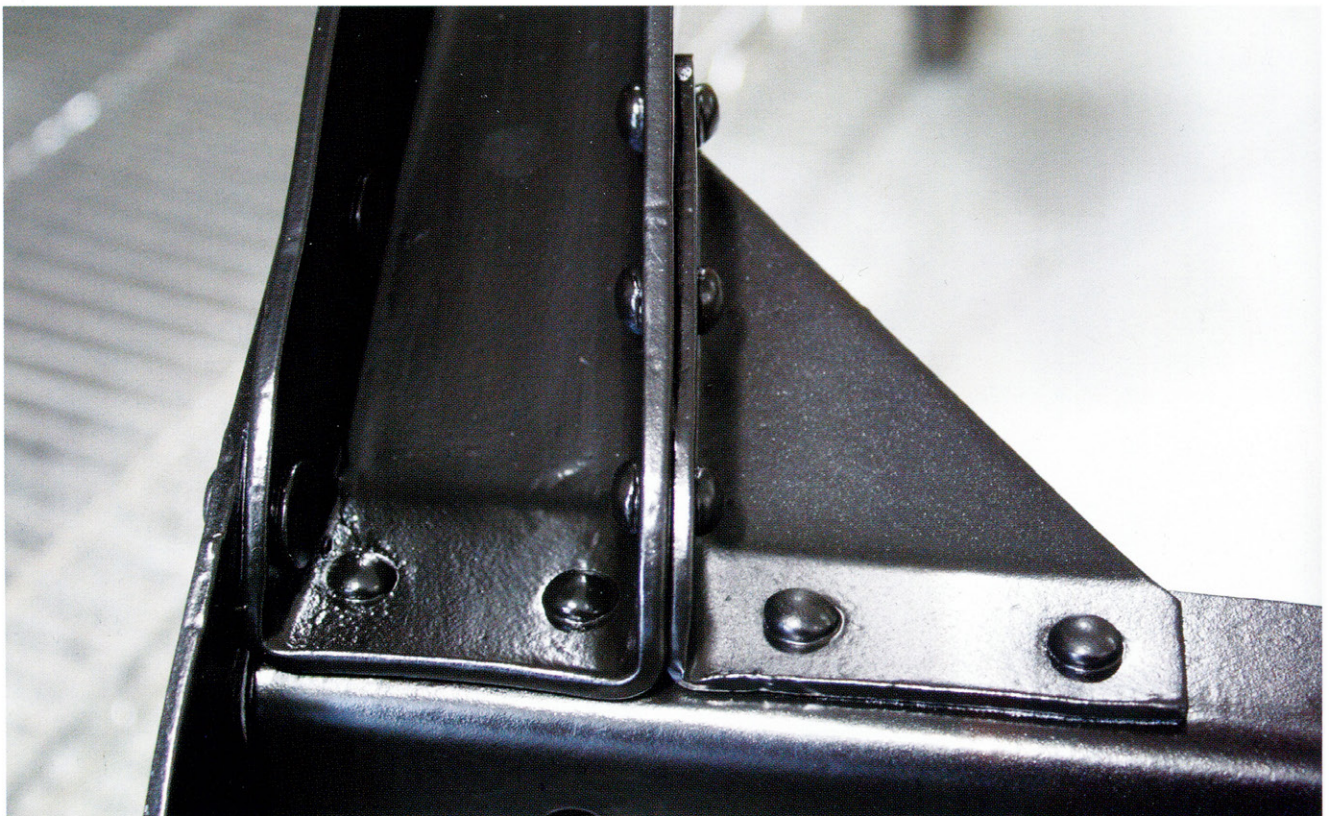
The rivets on this Ford Model T frame must have a certain appearance if they belong to a car that is being restored to like-new condition.
