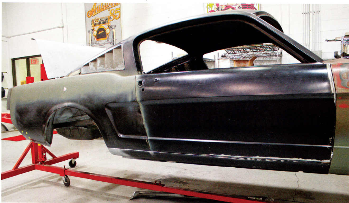
The relationship of the panels on the right side of this Ford Mustang look really nice, but it wasn't always this way. The clean lines and even panel gaps are artificial constructions created by the restorer looking for tasteful over-restoration.
