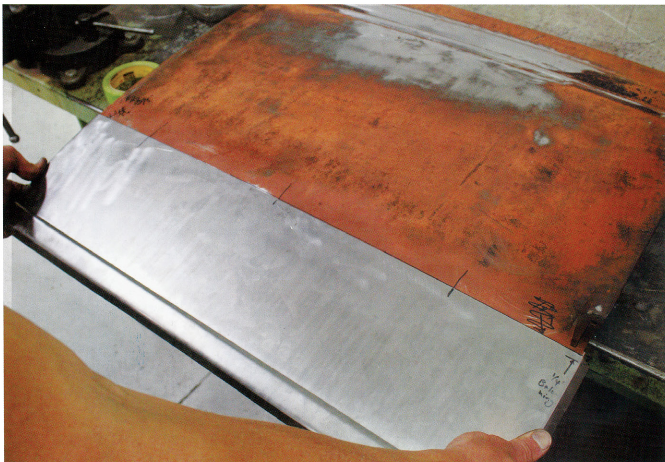
Besides a nasty karate chop across the belt line and some rust along the bottom, Joe McCullough's Model A door was fine. After a couple of tedious hours pushing inside the door with a dolly and tapping on the outside with a hammer, the belt line dent was repaired. The new skin was basically a crowned panel with a bead rolled along the bottom.
