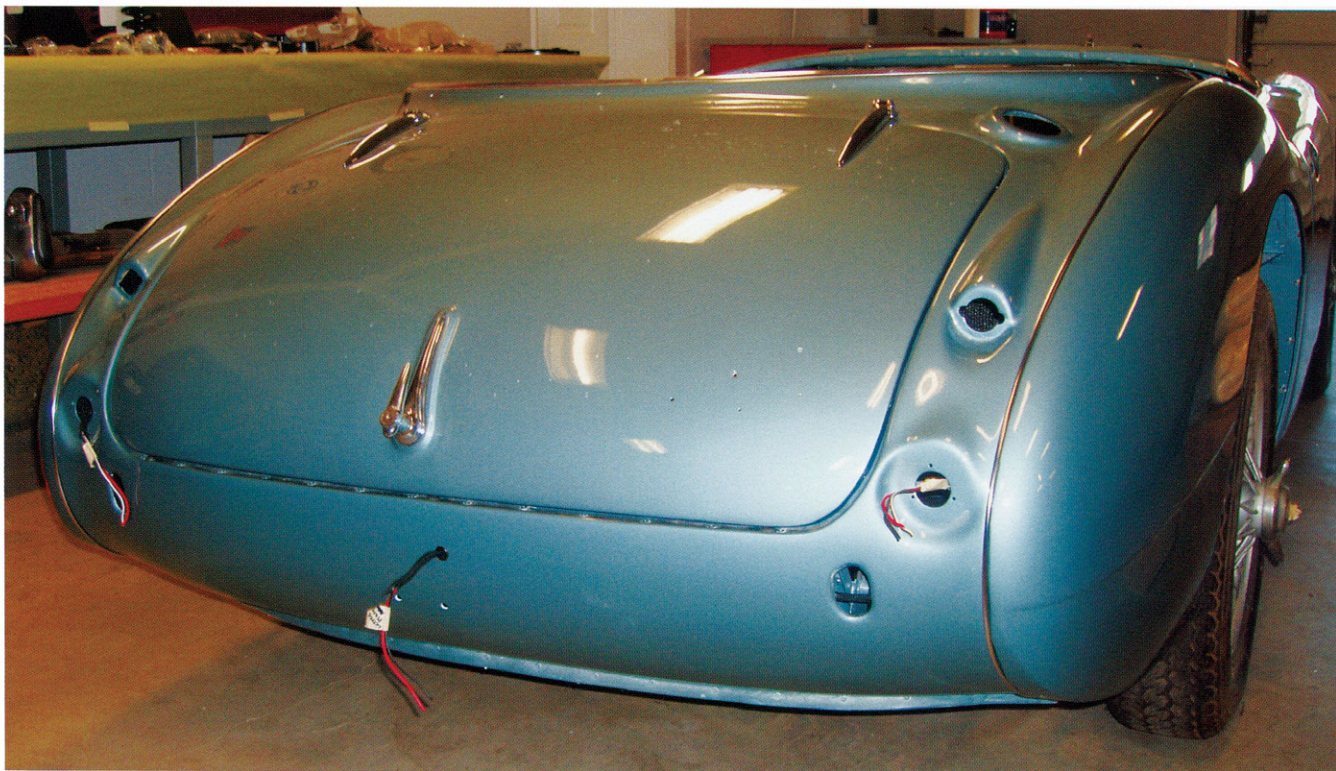
No one would ever guess that the lower third of this Austin-Healey boot lid was a rusty, perforated disaster a few months prior. With the help of a hand-shrinking machine, fabricating a repair patch was not difficult.
