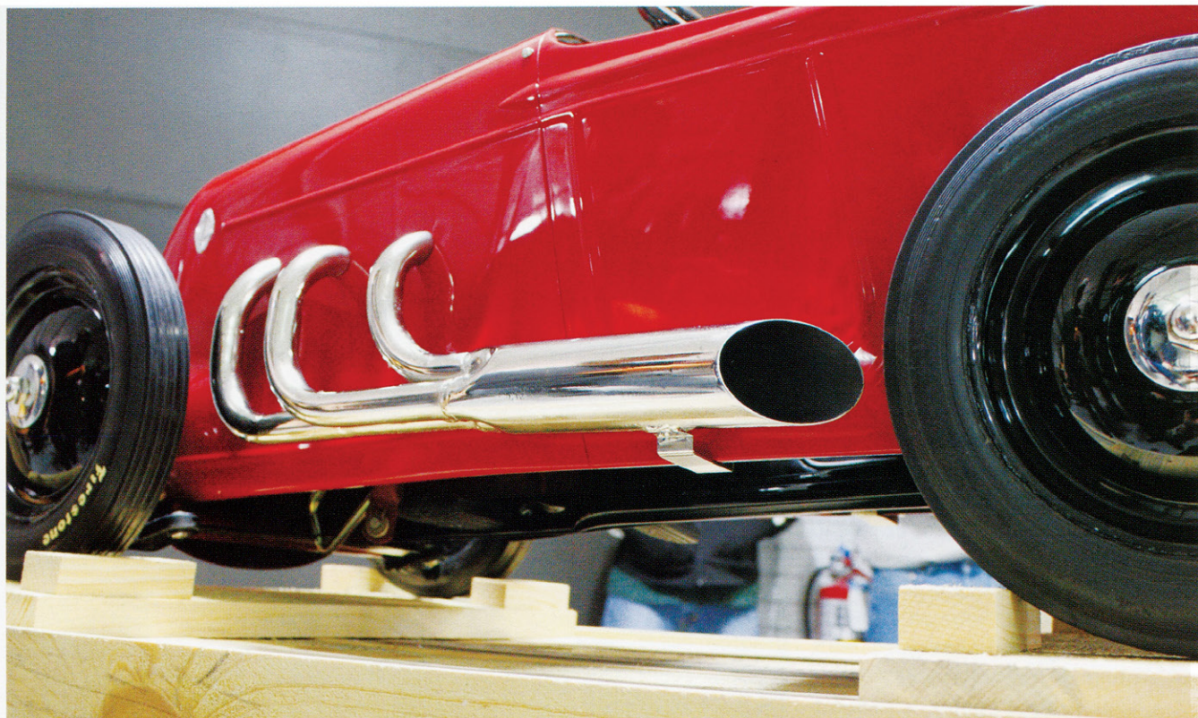
It is hard to believe that this pedal car header was made out of rusty bicycle handlebars and a length of automotive exhaust pipe. The transformation involved some welding, sanding, polishing, and nickel plating.
