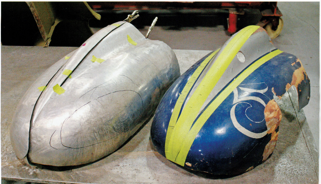
Lance Butler decided to recreate this tattered Kurtis-Kraft quarter midget tail section in aluminum. It's still a work in progress, but it suggests that great potential shaping projects are out there if you look for them. Lance borrowed the original from a guy he met at a swap meet.
