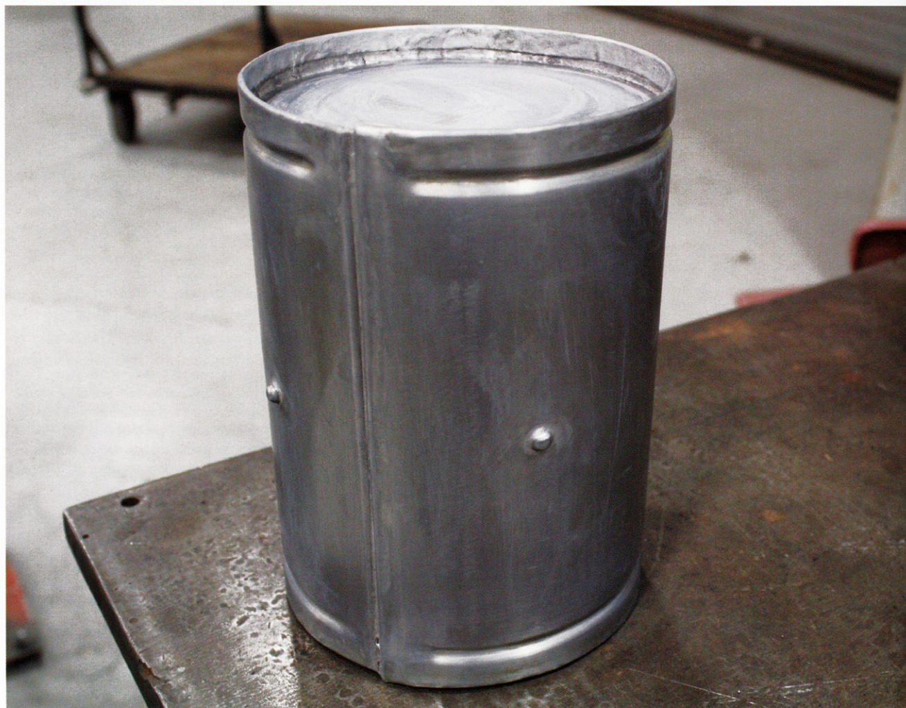
I made a gas tank similar to this for our engine dyno, but its construction is exactly as you might expect to find on an antique car. The skills needed to build it are a perfect culmination of material covered in this book thus far.
