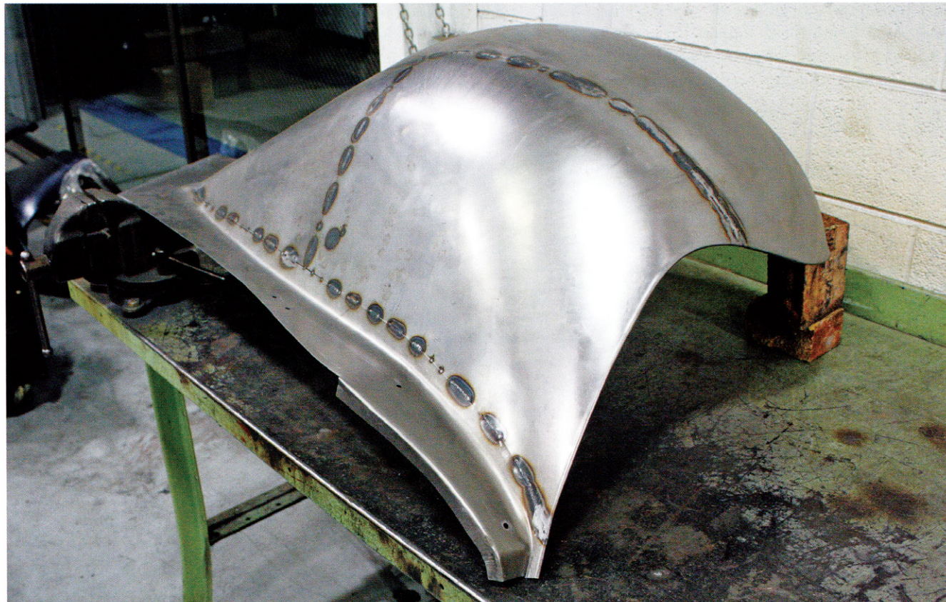
This fender seems complicated, but it is made up of eight individually shaped panels that were less intimidating when conquered one at a time following John Glover's classic video on the subject.
